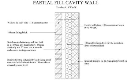
Fig. 11 Partial fill cavity wall (Not to Scale)
