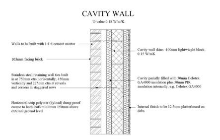
Fig. 7 Partial fill cavity wall with internal insulation (Not to Scale)
