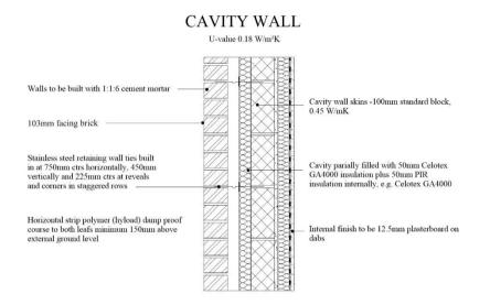
Fig. 15 Partial fill cavity wall with internal insulation (Not to Scale)
