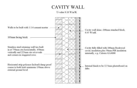
Fig. 14 Full fill cavity wall with internal insulation (Not to Scale)
