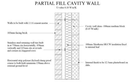
Fig. 13 Partial fill cavity wall (Not to Scale)
