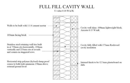
Fig. 2 Full fill cavity wall (Not to Scale)
