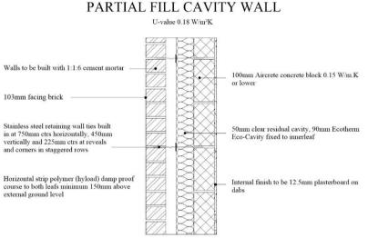
Fig. 4 Partial fill cavity wall (Not to Scale)
