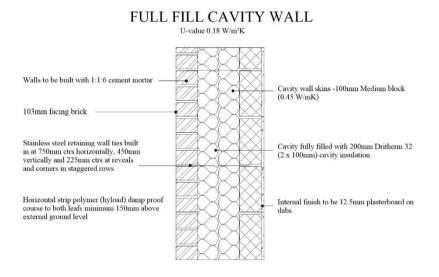
Fig. 8 Full fill cavity wall (Not to Scale)
