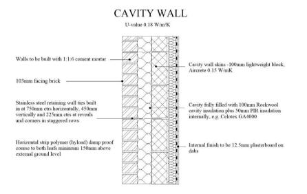
Fig. 6 Full fill cavity wall with internal insulation (Not to Scale)
