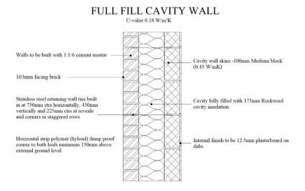
Fig. 9 Full fill cavity wall (Not to Scale)
